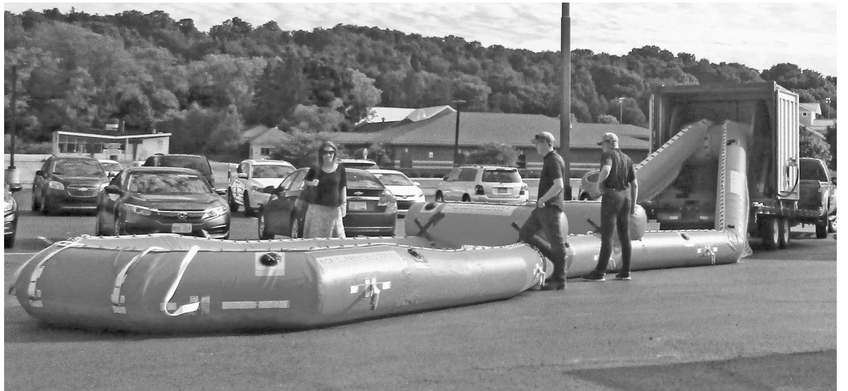
A team from Canadian-owned Enbridge Energy hosted a series of open houses throughout northern Michigan last week to showcase some of the $7 million in pipeline safety equipment it plans to acquire over the next two years. A NOFI Current Buster, pictured above, resembles an inflatable slide but actually is a device that can be towed through an oil slick and using high speed skimming technology, can rapidly recover oil in the back.
